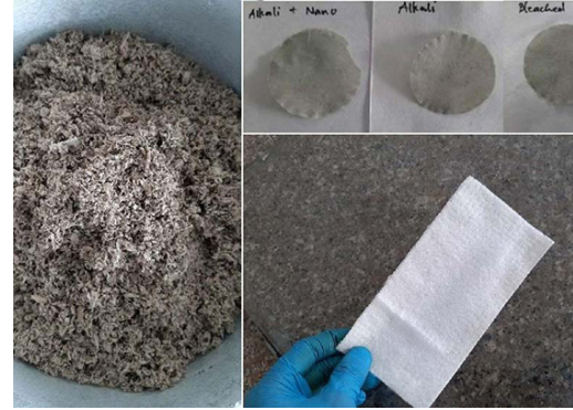
Caraga State University Nanocellulose films for face shields, disinfectant tents, aerosol boxes
